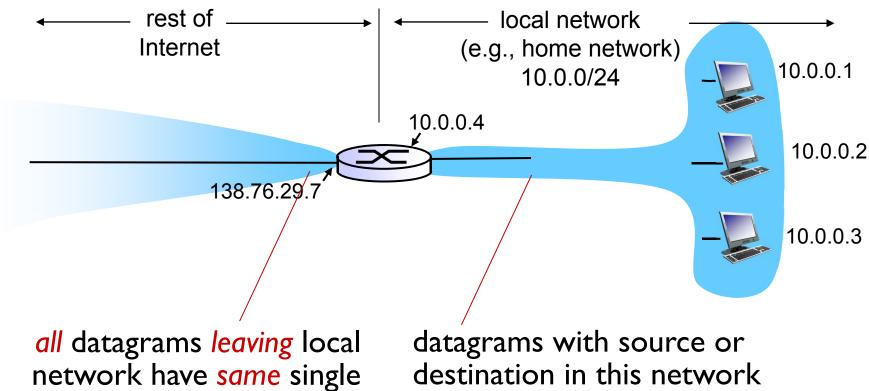
source NAT IP address: I 38.76.29.7,different source port numbers datagrams with source or destination in this network have 10.0.0/24 address for source, destination (as usual)
