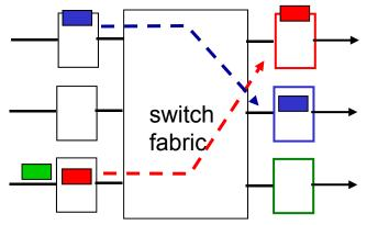
output port contention: only one red datagram can be transferred. lower red packet is blocked one packet time later: green packet experiences HOL blocking
