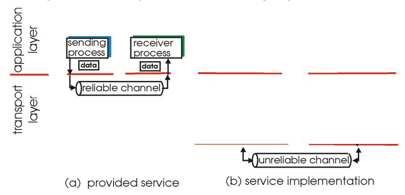
characteristics of unreliable channel will determine complexity of reliable data transfer protocol (rdt)
