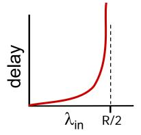
large delays as arrival rate, λ<sub>in</sub>, approaches capacity
